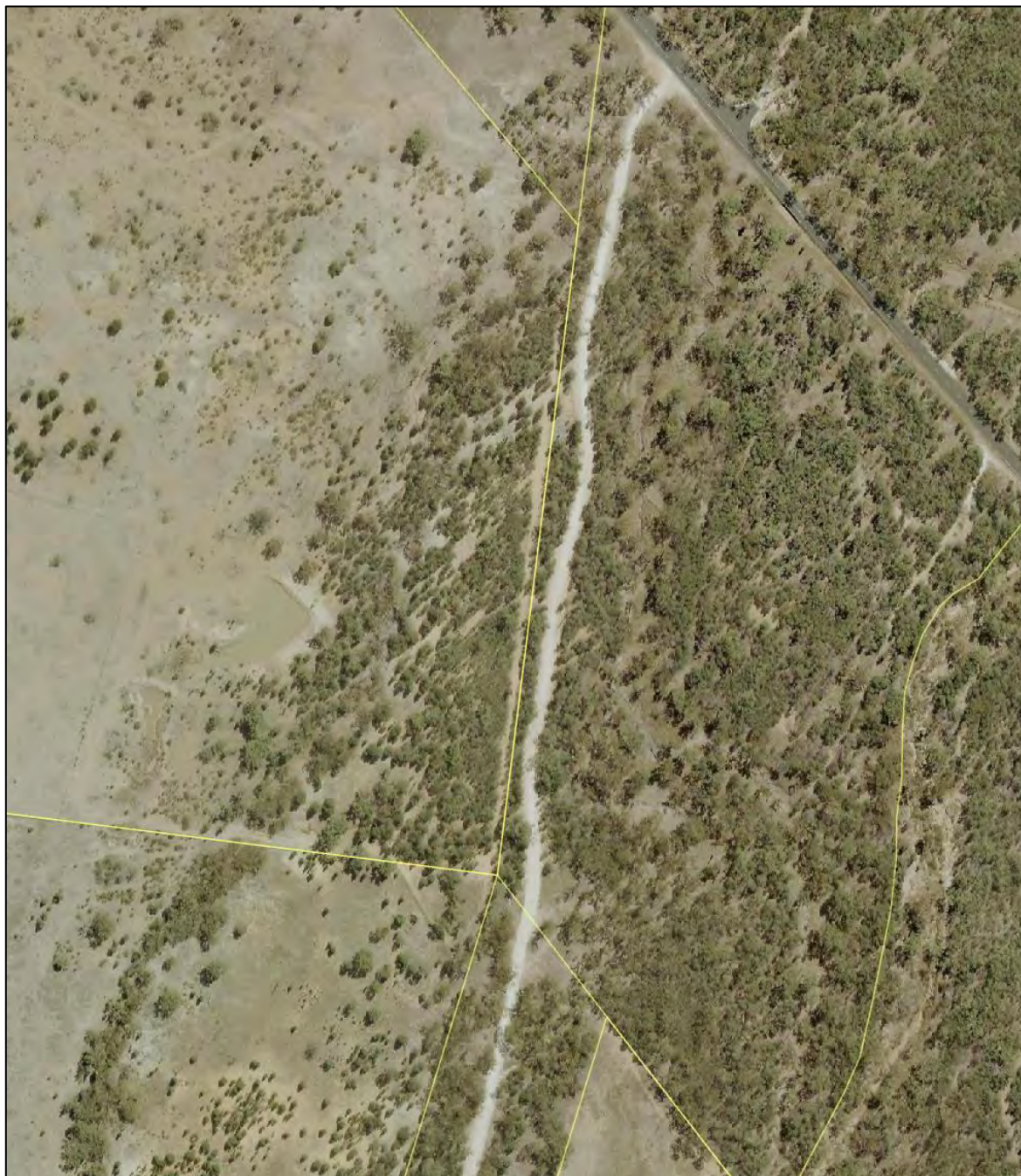
Figure 8: Substandard Horizontal Curves Between Access and Kogan Condamine Road (Aerial: QldGlobe)
